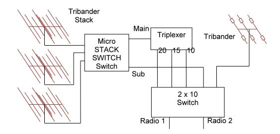
The triplexer allows both stations to use the same antennas.
