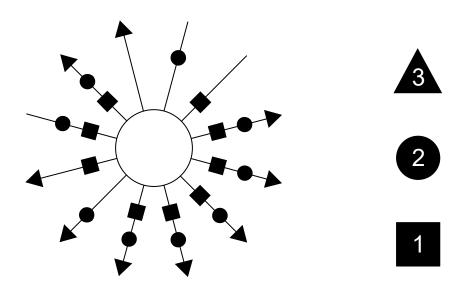
This scheme shows *exclusive antennas*. Each position selects an exclusive combination of antennas. (There are several positions which select all antennas because the switch they used had 12 positions).
