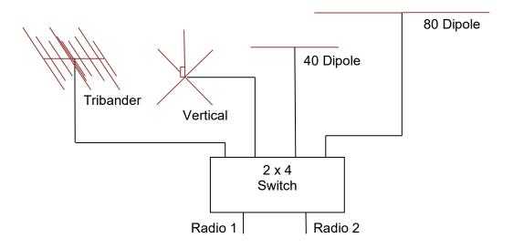
The Swap function has also been configured for this station. When selected on either station it will swap the antennas. It is only available if the antennas can actually be swapped. It is useful if one station is using the beam and one is using the vertical and the operator finds a pile-up on the vertical that he needs the beam to break.
