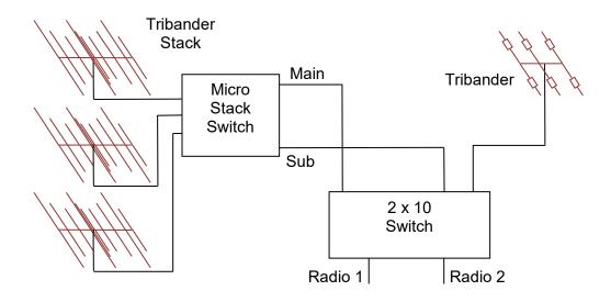
This switch is different than the common stack match because it has two feeds. The main feed has an impedance matching transformer and can connect to one, two, or all three tribanders. The sub feed has no matching network and can connect to one antenna at a time.
