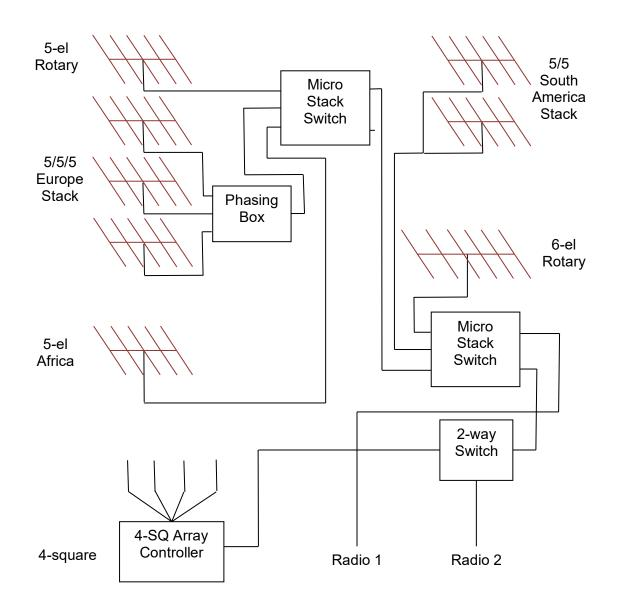
This is configured as one station with two radios to make it easy to demonstrate it using one copy of a logging program. Normally it would be two stations, each with one radio. This is a simple thing to change in the Stations list in the configuration file.
