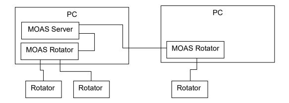
There is no practical limit on the number of computers running MOAS Rotator or on how many rotators are connected to each computer.
