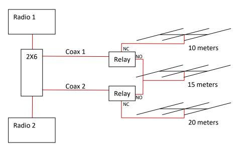
Since the two paths to the 15 meter antenna use different relays the MOAS server considers them to be different antennas. The configuration file specifies that they are alternates for each other and the server will automatically switch the 15 meter antenna path as necessary.
