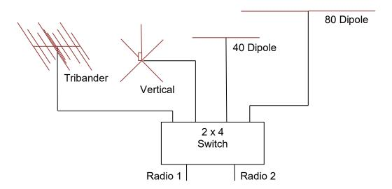
The Swap function has also been configured for this station. When selected on either station it will swap the antennas. It is only available if the antennas can actually be swapped. It is useful if one station is using the beam and one is using the vertical and the operator finds a pile-up on the vertical that he needs the beam to break.
