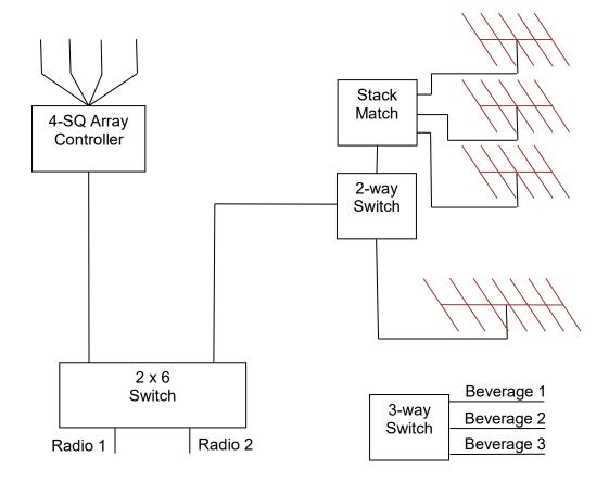
The beverages show antennas which are receive-only. It is not necessary to press the RX button before selecting one.
