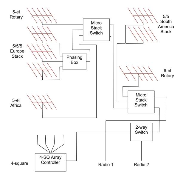
This is configured as one station with two radios to make it easy to demonstrate it using one copy of N1MM Logger. Normally it would be two stations, each with one radio. This is a simple thing to change in the Stations list in the configuration file.
