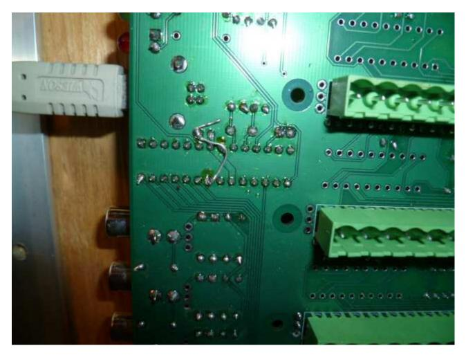
There is a hole provided to bolt Voltage Regulator U3 to the board. It is not necessary to install a bolt but if you want to you will need a #4x1/4" bolt, lock washer, and nut. Those parts are not on the parts list bur are available in any hardware store.
