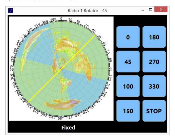
No short heavier line is shown because there is no rotator for this fixed antenna.
