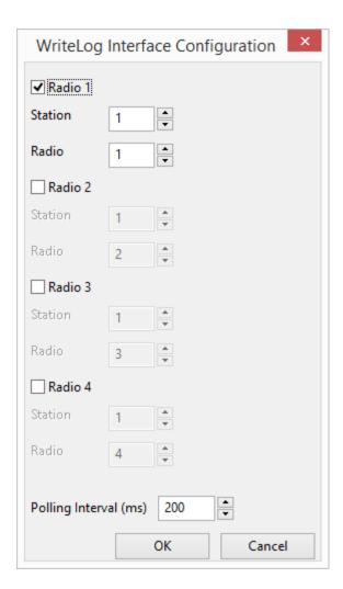
The polling interval controls how often the client checks the frequencies in WriteLog. A longer polling interval reduces computer overhead but will increase the time between changing bands and the server changing antennas.
