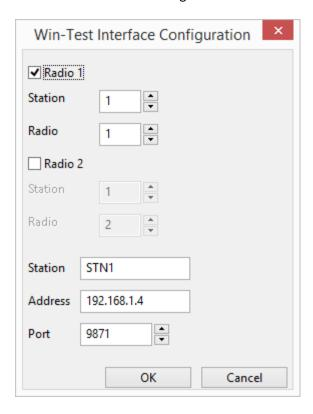
The address should be the address of the computer which is running Win-Test.
