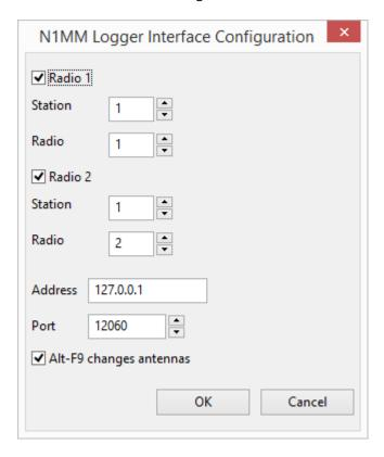
Use only Radio 1 or SO1R or SO1V. Use Radio 2 for SO2R when the logging program is controlling two radios.
