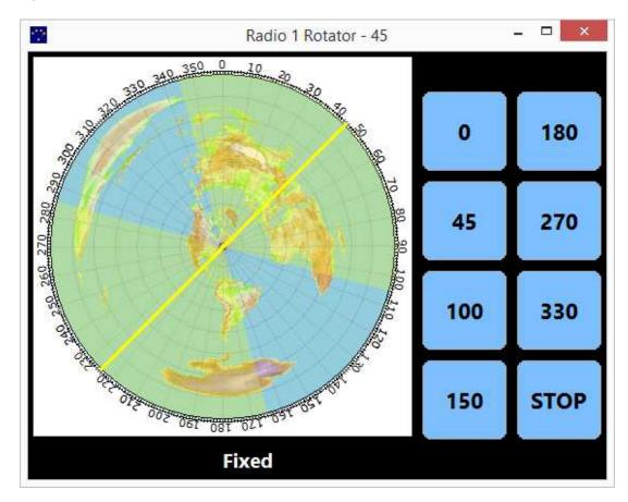
If a no rotatable antennas fit the selection then a fixed antenna can optionally be shown. This is a fixed dipole which is a bidirectional antenna.
