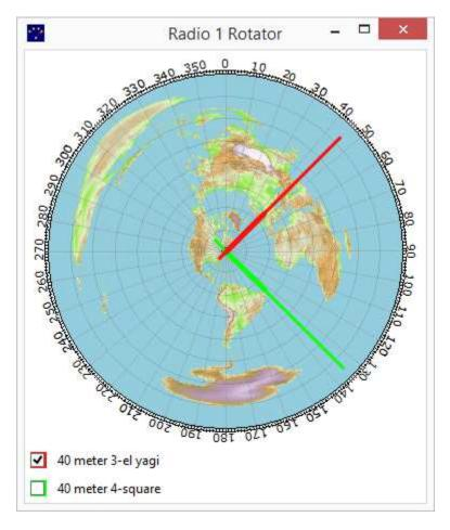
Clicking on the compass will rotate the yagi but will not change the 4-square because the yagi's box is checked and the 4-square's is not.
