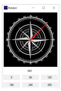
Scripting will be used to select antennas and rotate the triband beam using the keyboard. The script shows the use of the commands to select an antenna and activate a function in a display window and to set a rotator direction.
