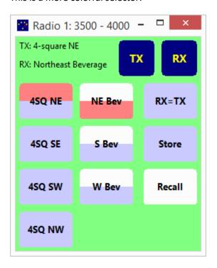
The selected antennas are the 4-square NE for transmit and the NE Beverage for receive. RX=TX is available.
