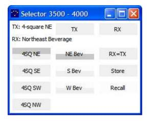
The Antenna Selector can show the transmit / receive status of the radio if the server is configured to do this. It will also indicate that the radio is inhibited and cannot transmit and that the server is not able to communicate with the switch. This is done by changing the color of the window background or of the background behind the antenna name.
