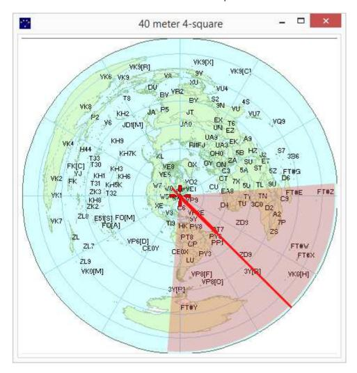
Since the 4-square is electrically rotatable the direction can be changed by turning the rotator in a Rotator Direction window or by selecting one of the four antennas in an Antenna Display or Antenna Selector window.
