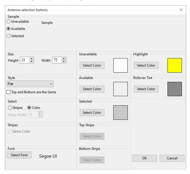
Select **Unavailable**, **Available** or **Selected** to set the sample button to the antenna unavailable, antenna available, or antenna selected state.
