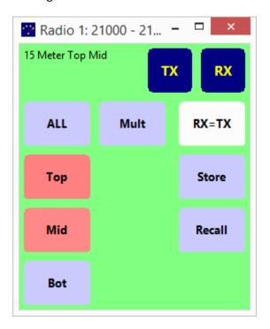
Pressing the ALL button or pressing the Bot button will cause all three antennas to be selected:
