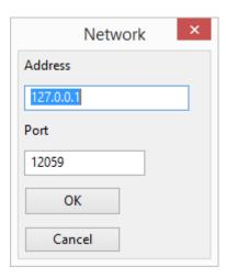
If the server is running on the same PC as the client then the default address will probably work. Otherwise it must be the IP address of the PC that is running the server.
