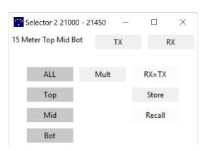
This script is more complex than the simple station script. The behavior of the keys depends on the band and which antenna is selected. Pressing a key multiple times can switch between antennas or can activate or deactivate a receiving antenna.
