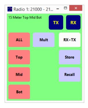
If a single antenna from the stack is desired the other two could be clicked to deselect them. Alternatively the window can be configured so that double-clicking or right-clicking a button will select that antenna exclusively and will deselect all others. On a touch screen a touch and hold can also do this.
