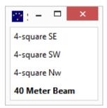
In this case the window is configured to show a maximum of four antennas. There are five antennas available on this band so one is not shown. The list will be shifted if necessary so the selected antenna will be shown.
