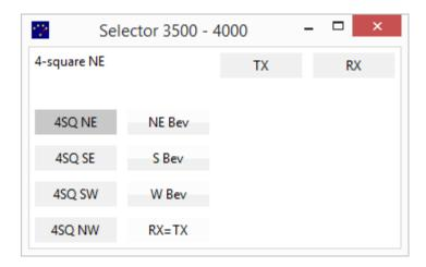
The selected antenna is displayed in the upper left corner. There are TX and RX buttons which are used to change only the transmit or receive antennas. These items can be configured as desired.
