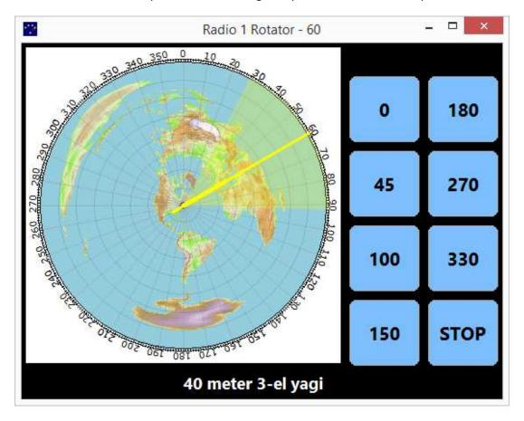
The button presets are configurable. Any direction can be placed on a preset.
