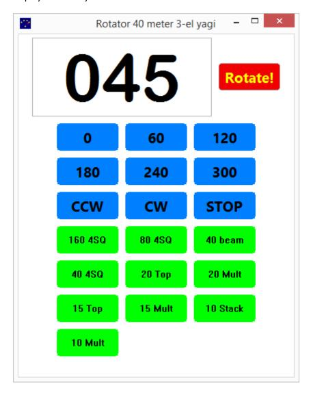
Typing a number into the box and pressing the Rotate! button or pressing the Enter key will cause the rotator to turn to the specified direction.
