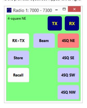
The Antenna Selector can be run on any PC that can connect to the server. The only restriction is that if it is not on the same PC as the logging program it cannot display the antennas for the radio with logging focus.
