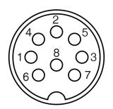
This view shows the connector pin numbering as seen looking at the back of the SO2R Box (plus). Note that the pins on a DIN connector are not numbered sequentially.
