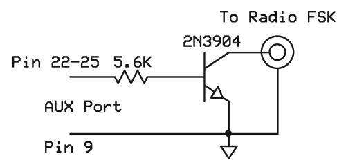
The disadvantage of a single-transistor interface is that the grounds of both radios are connected to pin 9 of the AUX connector and to the SO2R Box (plus) ground. This could cause a ground loop.
