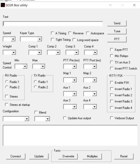
The SO2R Box utility program allows access to SO2R Box (plus) features without using a logging program. It can be used to test the box and also to load new firmware.
