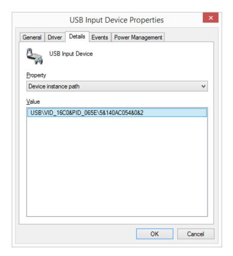
If you are able to find the SO2R Box (plus) HID device in Windows, then Windows has loaded the necessary drivers and is communicating with the SO2R Box (plus). Check the Details tab and select Device Instance ID in the menu. The information shown should start with USB\VID\_16C0&PID\_065E. If the numbers you see do not match these, the firmware is probably corrupt. Try to re-install the firmware using the Programming Jumper as described in Chapter 7.
