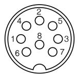
This view shows the connector pin numbering as seen looking at the back of the SO2R Box (plus). Note that the pins on a DIN connector are not numbered sequentially.
