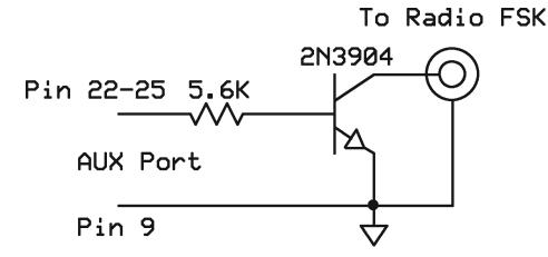
The disadvantage of a single-transistor interface is that the grounds of both radios are connected to pin 9 of the AUX connector and to the SO2R Box ground. This could cause a ground loop.
