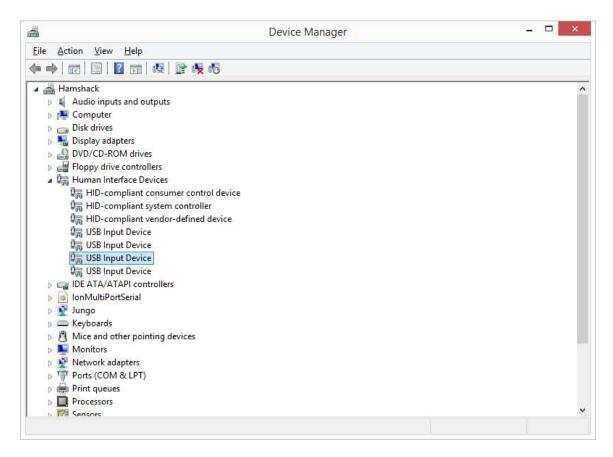
The SO2R Box (plus) is a USB Human Interface Device. Some versions of Windows will show it as an input device. Double-click on them one at a time until you find a box that says it is for the SO2R Box. The device properties window should look like this:
