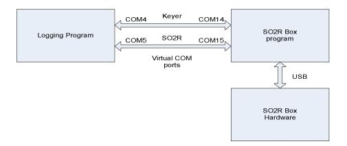
This diagram shows how everything communicates. The port numbers are set up in the configuration utility of VSP Manager, com0com, or vCom. The port numbers in the picture were chosen because they work with N1MM Logger, Win-Test, and WriteLog, but you can use any port numbers except the ones already assigned to other ports on your computer.
