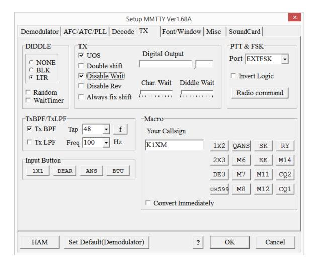
The right side of the dialog has a drop-down menu labeled PORT. Select EXTFSK. This item is at the bottom of the list, below all the COM ports.
