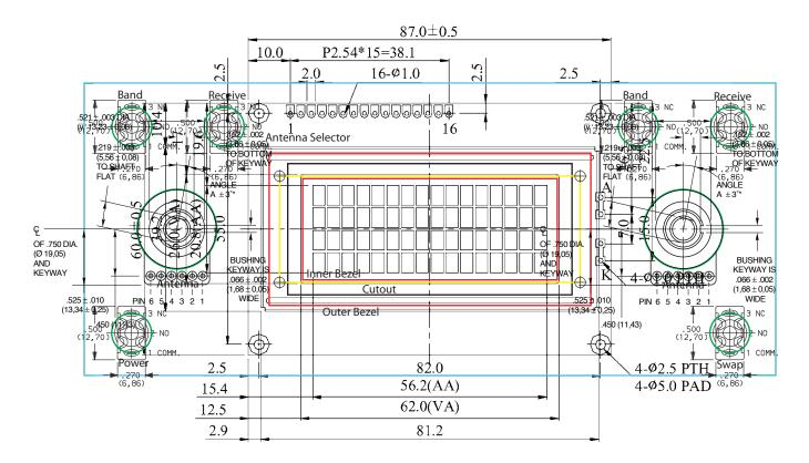
Front Panel sized for Ten-Tec TPB-45 2.75" x 6.5" box Encoder knobs are .75" Pushbutton knobs are .375" On/Off switch is drawn as pushbutton
